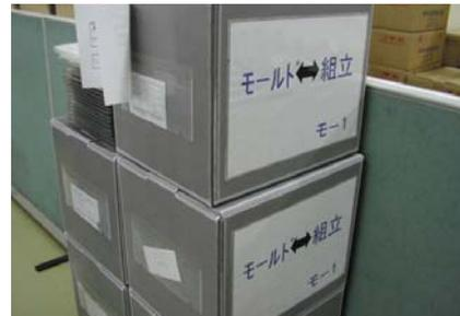
Foldable containers used to transport molding parts within the company
