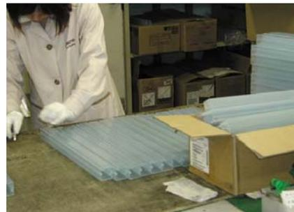
Plastic trays and stick packing trays are inspected and sorted for reuse
