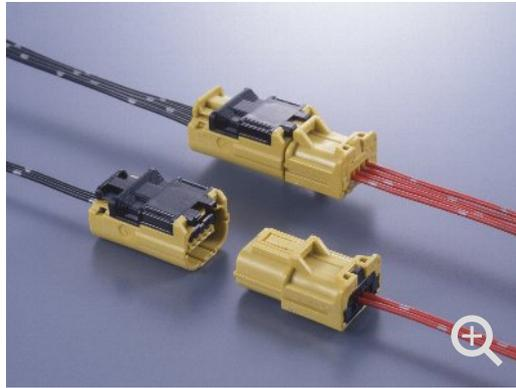
The MX36 Series waterproof compact inline relay connector was developed for use with automotive airbags. It features a structure that separates the connection of the contacts with the repulsion of the air spring when the connectors are not completely mated (mechanical perfect mating design). Waterproofing performance is accomplished with the rubber sealing ring of the mating portion and the grommet rubber on the wire.
