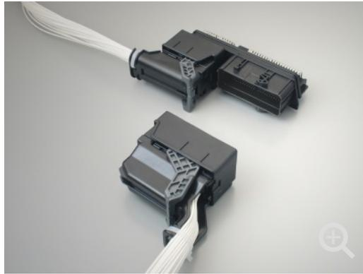
An automotive grade waterproof connector ideal for engine compartment applications has been developed. Compatible with a high pin count of 177 positions, it features a lever structure and downsized contacts that reduces operation force.
