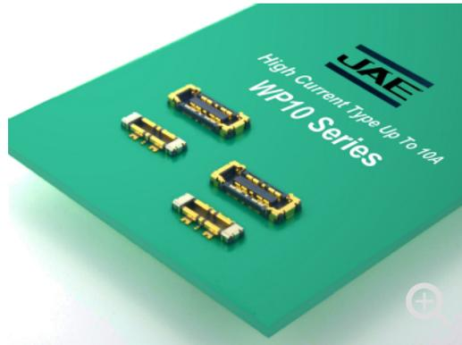
The WP10 Series is a stacking type board-to-board(FPC) connector which is low-profile and saves space. It is ideal for high-current connection areas like battery connections in compact hand-held devices such as smartphones, wearable device and tablet PCs.
