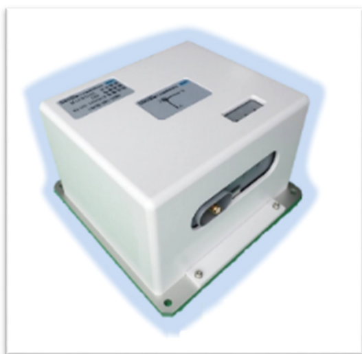
Figure 7. External view of RTK positioning-IMU prototype model
