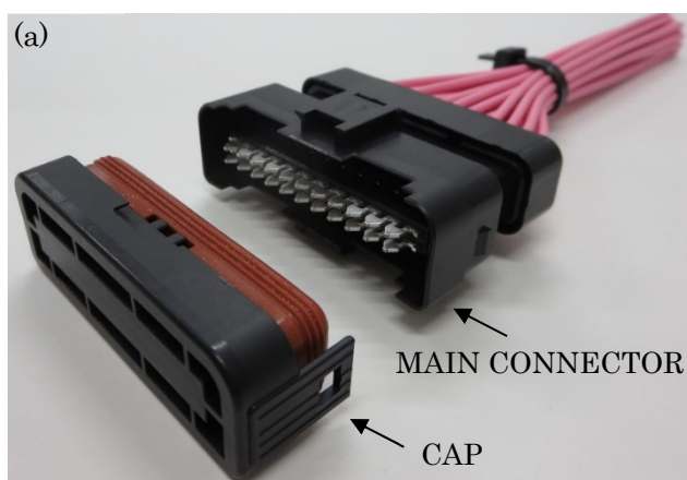
Fig.1 HB07 Connector overview (a) Cap released, (b) Cap attached
