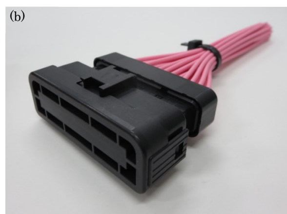
Fig.1 HB07 Connector overview (a) Cap released, (b) Cap attached
