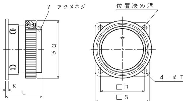
Box shaped receptacle with socket insert.
