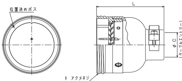
Straight plug with pin insert.
