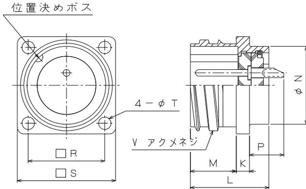
Box shaped receptacle with pin insert.
