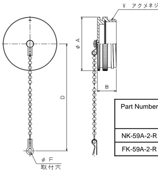
Used to protect mating surface, keeping out dust and other foreign substance, and to prevent danger caused by electrical circuit of disengaged connector mating surface.
