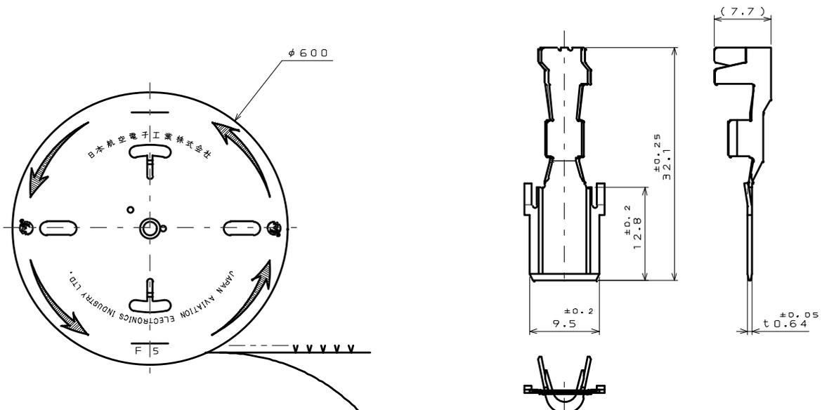
PW01-PC1-2-\* -800E Magazine assembly (Pin contact)
