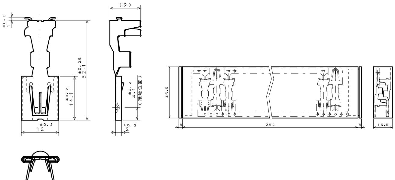
PW01-PC1-\* -800E Magazine assembly (Pin contact)
