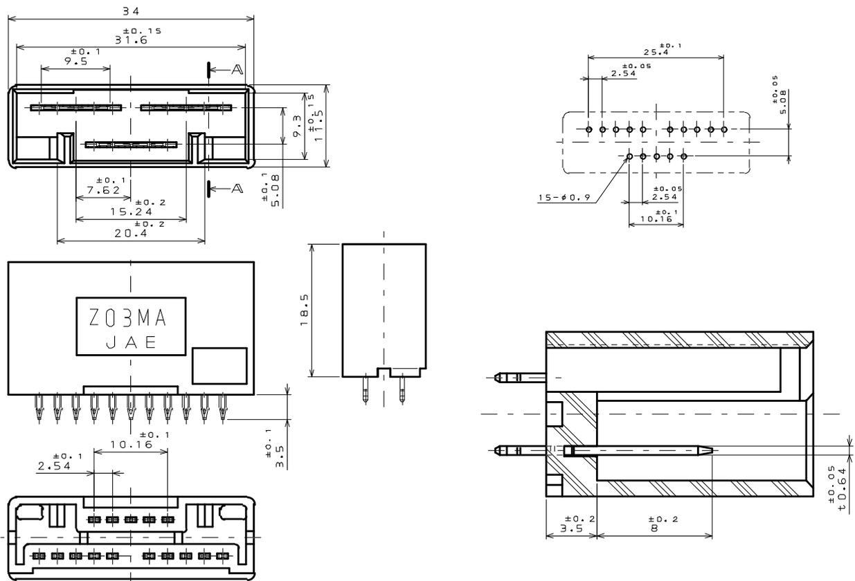
PW01-3PC-A\* Insulator (3pos. Connector for electric wire relay)
