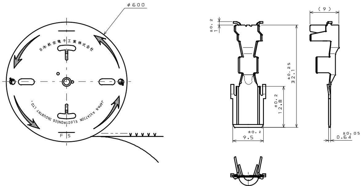
PW01-PC1-1-\* -800E Magazine assembly (Pin contact)
