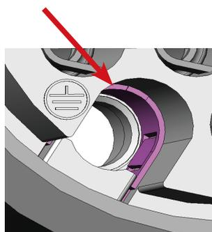
Grounding lug to connect contact to outer metal shell
