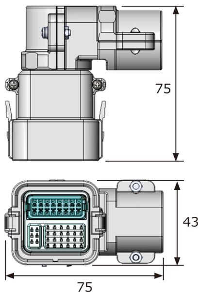
Angle plugs can be set to eight directions in 45° increments
