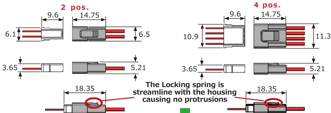
Compact and streamline housing allows for passage through narrow spaces, such as inside a robot arm.
