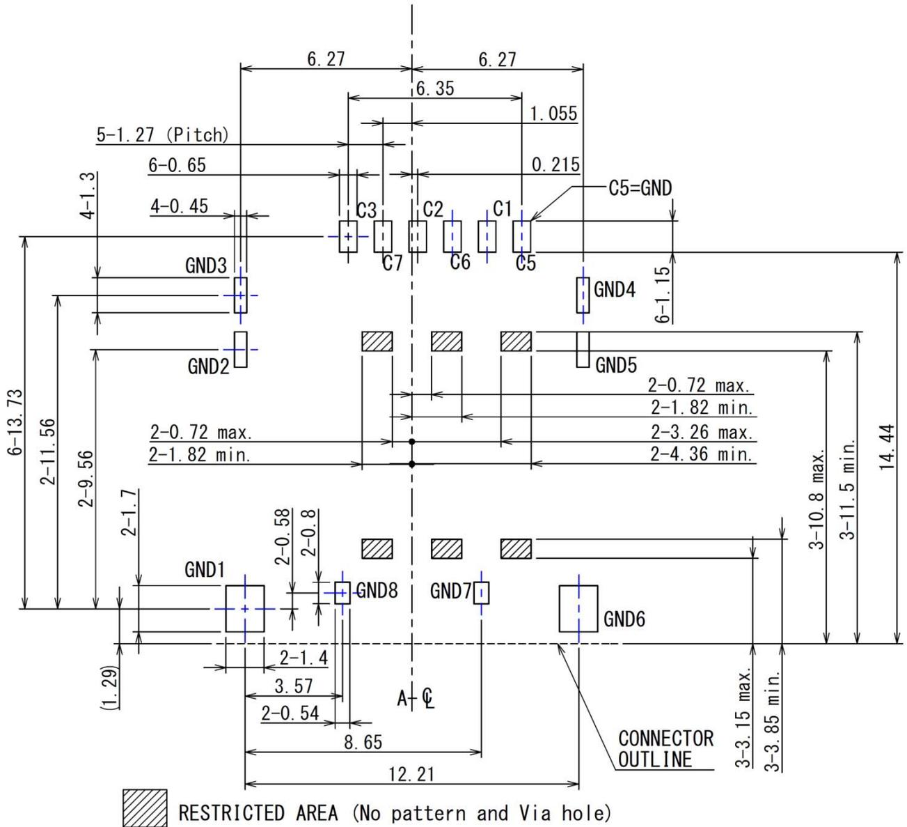
All patterns and Via holes under the connector should be coated by resist.
