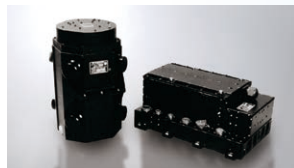
Inertial sensor unit for rockets
